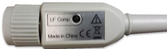
Figure 2. Low-frequency compensation adjustment (for N2840A/41A/42A/43A/53A)
